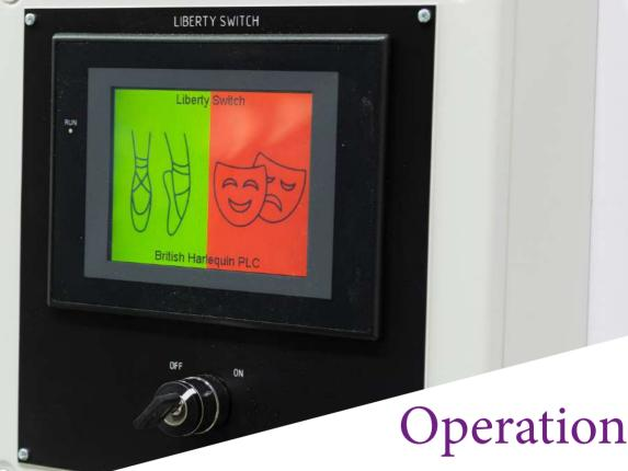
Harlequin Liberty Switch is very simple to operate. The system is controlled remotely via a hard-wired master control unit which can be integrated with most existing stage control or building management systems.
