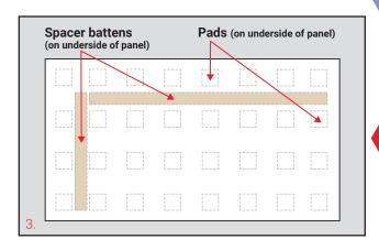
Place 12mm packers between the wall and the panel, two on the long edge and two on the short edge. (See diagram 4). This will create an expansion gap and will help to keep the panels square within the room. Skirting can be installed when the floor is complete (once the packers are removed) to cover this gap if desired.
