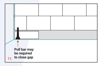
Lay the remaining panels of the last row as above. Note that the final panel will probably need to be cut on two edges and will require 12mm packers between the panel and both walls. If glue has been used, leave the packers in place until the glue has set, then remove them. The floor joints may require sanding to remove surplus glue before the top surface is laid.
