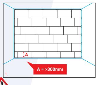
It is critical that the first row is laid accurately. If it is not straight the floor will be out of alignment.
