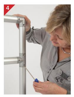
**4.** Tighten the hex screws with the Allen/hex key provided.
